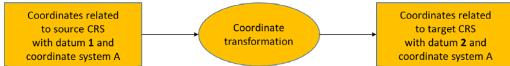
Figure 30: Process flow diagram for a coordinate conversion (based on Ihde et al., 2012)
