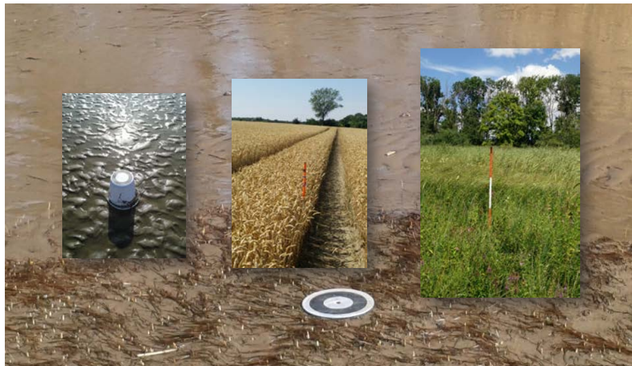
Figure 71: Ground control points for every situation
