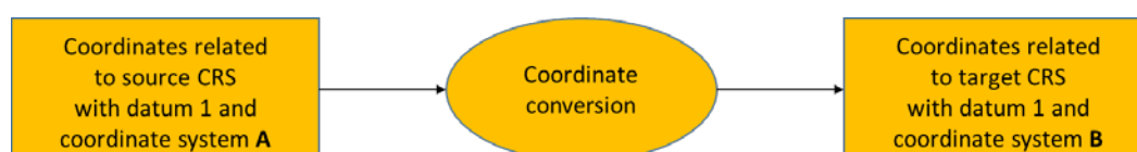
Figure 29: Process flow diagram for a coordinate conversion (based on Ihde et al., 2012)
